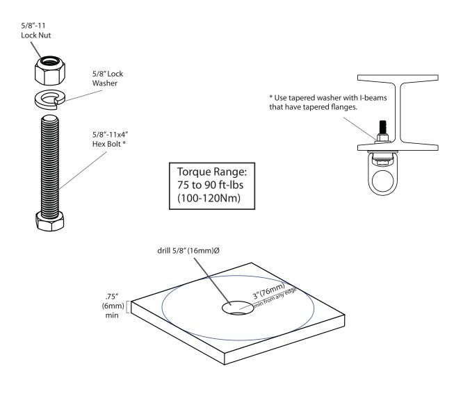
\* For steel applications a grade 5, grade 8 (or equivalent) bolt no shorter than 4" (100mm) with a locking nut and washer must be used. Swivel anchor must be flush with steel surface. A 16mm bolt of equal strength may be used in place of a 5/8"-11 for metric applications.
