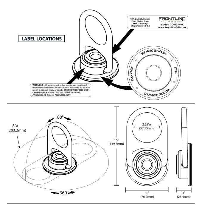
Tensile Strength (UTS): 10,000-lbf (44kN) Working Load: 2,000-lbs (907kg) Weight: 1.2-lbs (544.3g) Materials: Zinc Plated Steel Regulatory Compliance: Meets or exceeds ANSI Z359.18 Type A, ANSI Z359.7-2011 OSHA 1926.502
