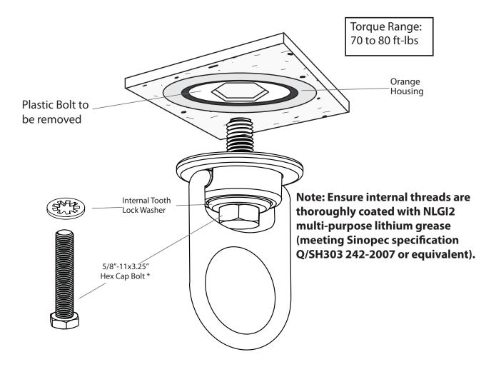
WARNING: Do not install if insert was knocked over during installation. Mega Swivel must mount flush to surface when fastened with the proper torque.
