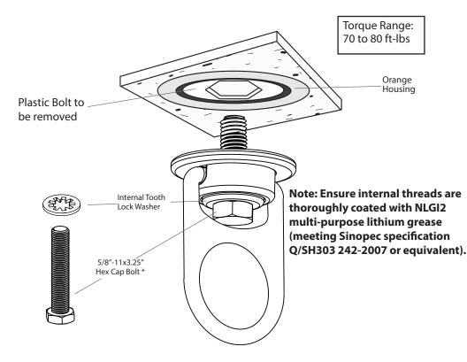
WARNING: Do not install if insert was knocked over during installation. Mega Swivel must mount flush to surface when fastened with the proper torque.
