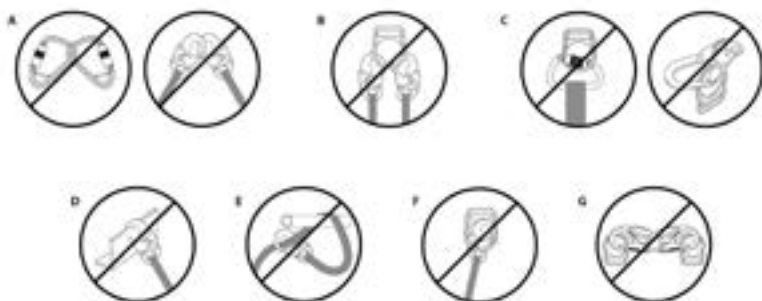
Figure 4 - Raccordements non compatibles
