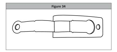
Step 5: Inspect the Ratchet Strap Tensioner webbing for cuts, fraying, and signs of damage from excessive wear or abrasion. Also check for excessive dirt, grease, oil, paint, or other surface contamination or discoloring. Check all stitch locations to ensure that each is intact with no loose, frayed, or torn threads.
