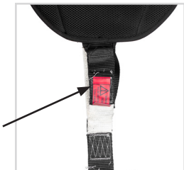
Red Exposed - Impact Indicator Broken - Remove From Service -
