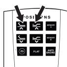
Then simultaneously press and hold HEAD UP and FOOT UP buttons. The remote backlight will flash. When lights turn off, remote should be sync'd. Test to confirm. Repeat if no function.
