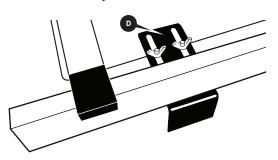
Connect the 4 brackets with wing nuts to the slotted plates in downward position as shown. Tighten wing nuts and make sure brackets are installed flush with the edge of foundation.
