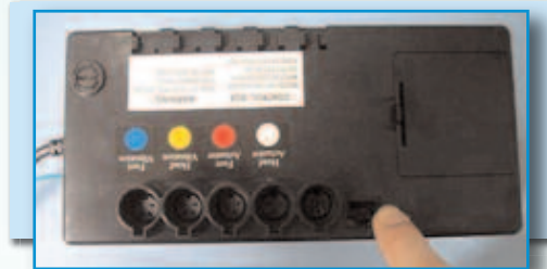
Figure 1: Press the "Learn Button" to initiate the RF learning mode.
