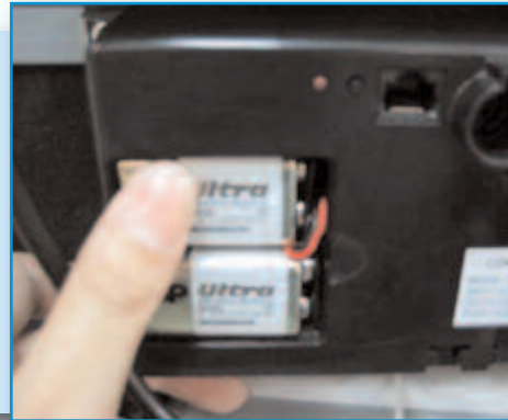
Figure 6: Install the 9 volt batteries
