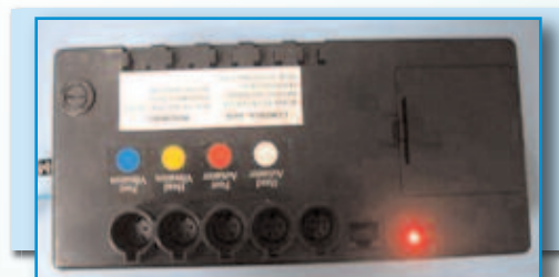
Figure 4: A flashing red LED indicates the control box has received the remote control figure
