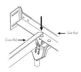
insert the glide **OR** roller into the sockets on all legs.
