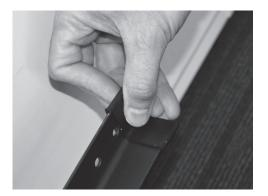
I-CS model frames have a double center rail. Insert a screw through the holes at the ends of the center rail and the two end holes in the side extender rail. Center rail should run head to foot. Secure with thumb nut. Repeat on the other end.
