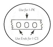
For I-PK model frames: Insert a screw through the hole in the center rail and the middle hole in the side extender rail. Center rail should run head to foot. Secure with thumb nut. Repeat at the other end. Center rail can be used for all sizes.
