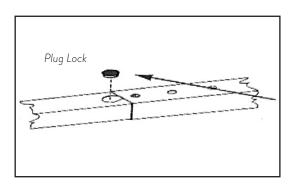
Attach each end of center rail to the extender rails using screws and thumb nuts. First, select the correct holes on the extender rails, which will be determined by your frame model. For I-PK frames, use just the center hole. I-CS frames use the first and third hole (not the center hole).
