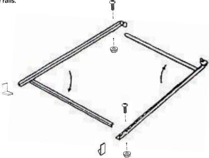
2. Secure the 4 strap braces to the side rails with the remaining nuts and bolts, and screw the threaded glides all the way into the legs until the pre-installed nuts are tight against the strap braces.
