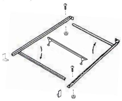
2. Secure the 4 strap braces to the side rails with the remaining nuts and bolts, and screw the threaded glides all the way into the legs until the pre-installed nuts are tight against the strap braces.
