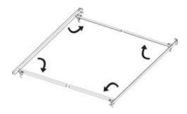
3 Insert 6 plastic sockets into legs on cross rails. Insert glides into plastic sockets
