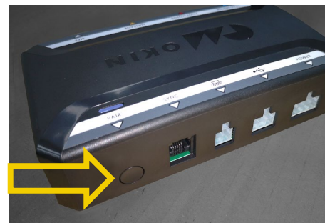
Option 2. Press the PAIR button on the control box twice.
