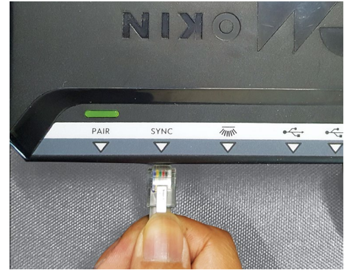
Connect the sync cable to the control box on both beds to operate them in tandem mode using the mobile app.
