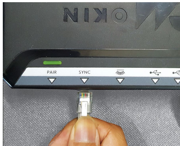
Connect the sync cable to the control box on both beds to operate them in tandem mode using the mobile app.
