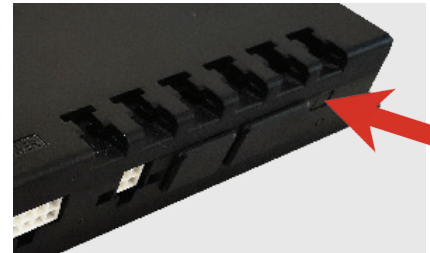
Learn button on the control box
