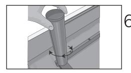
Insert the legs into the threaded holes at each corner of the base and rotate clockwise until tight. There must not be any gap or wobble in the leg in order to avoid risk of injury or damage to the base which may void warranty.
