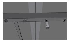
Secure the Base Pieces to each other using the eight hex bolts (four hex bolts for each Connecting Rod) making sure to hand tighten each and then tighten 1/4 turn more, as over-tightening could cause damage to the frame or Connecting Rod.
