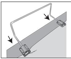
Remove the Mattress Retainer Bar from the bottom of the base. Finish removing the plastic packaging from the base to orient into final position. Carefully rotate the base on its side, then lift and place on legs. IMPORTANT: DO NOT LEAN THE BED AGAINST THE INSTALLED LEGS TO TURN OVER.
