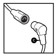
6 Insert DC cord from base into the power supply.
