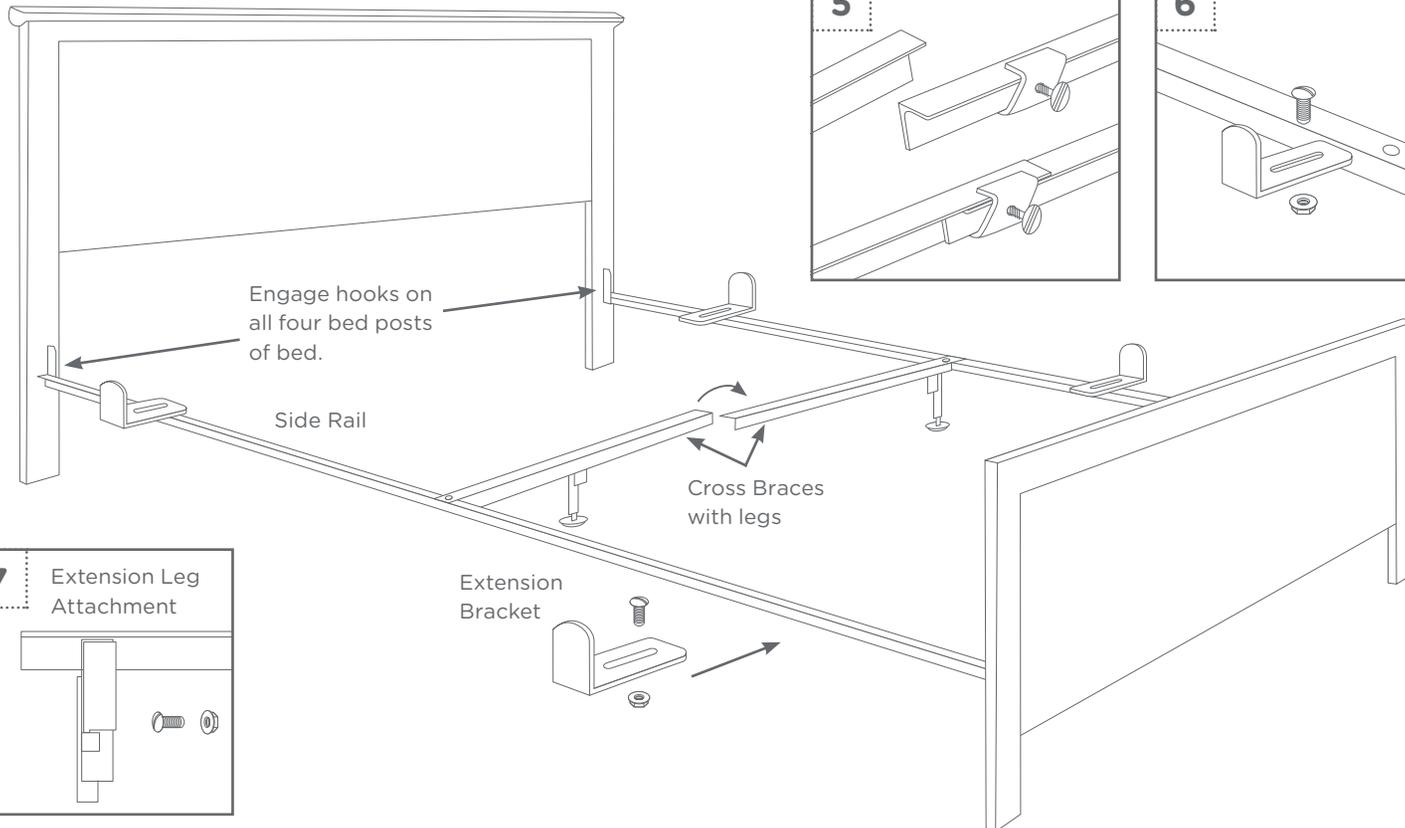
1. Engage hooks of rails in slots of headboard and footboard at full size position, with horizontal flange of rail protruding outward, as shown. Tap all hooks securely into slots of bed end.
