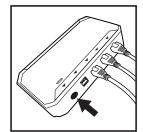
Double click the PAIR button on the control box (light will turn blue during the pairing process).
