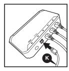
With both bases in FLAT position, connect each base to the other by inserting SYNC CABLE into each control box slot labeled sync.
