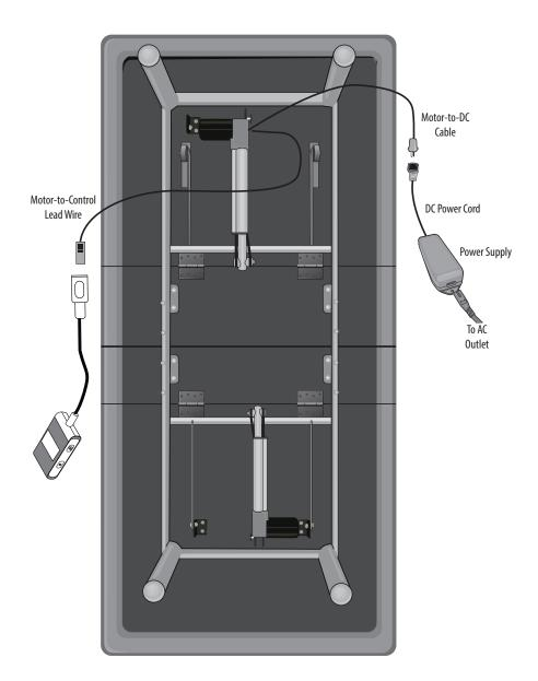
**NOTE:** Make sure wire connected to Power Supply is routed UNDER the main metal frame and lifting mechanism.
