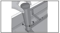
Insert the legs into the threaded holes at each corner of the base by inserting the leg and rotating clockwise until tight. There must not be any gap or wobble in the leg in order to avoid risk of injury or damage to the base which may void warranty.
