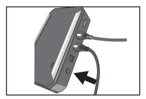
**USB:** This bed can charge standard devices that utilize a USB cable. A pair of USB jacks are located on each side of the bed base. Simply plug a USB cable into one of the USB jacks, and the other end into the device you want to charge.
