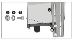
4 Put E through Part B and Part D. Then use H and G to fasten.
