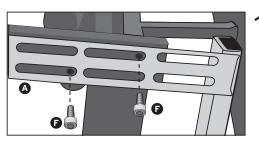
Remove the Mattress Retainer Bar from Align bracket A with holes running alongside base. Secure with 2 hex bolts F threading through headboard bracket mounting.
