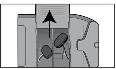
Turn the power supply upside down to access the battery cover, then slide the battery cover off.
