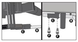
3 Insert part B into part C and secure with 2 hex bolts F.
