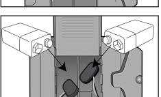
10 Insert the two 9V battery (included) into the compartment and slide the cover back on.
