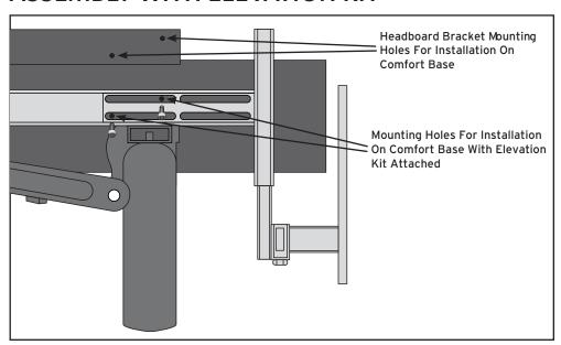
If attaching headboard brackets to a base with the elevate feature, please be sure to attach the brackets along the elevate kit. See image (location) to help locate the correct mounting location.
