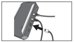
If setting two Twin XL's bases to use with one king size mattress, connect the Sync cable to the control box (as pictured) to one base. After bases are arranged, connect the second Sync Cable to other base's control box.
