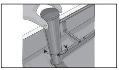
Insert the legs into the threaded holes at each corner of the base by inserting the leg and rotating clockwise until tight. There must not be any gap or wobble in the leg in order to avoid risk of injury or damage to the base which may void warranty.
