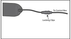
Insert one end of the DC cord into the power supply. Insert the other end with locking clips into the Control Box. Lock the Control Box using the locking clips.
