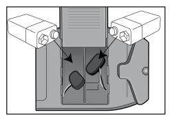
10 Insert the two 9V battery (included) into the compartment and slide the cover back on.
