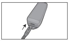
**?** Insert the AC cord into the power supply.
