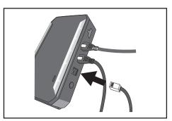
$3 \ \, \text{Insert the foot motor cable into the} \\ \text{Control box}.$
