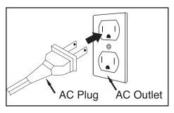
14 Insert AC plug into an AC outlet having 100-240V AC, 50/60Hz.
