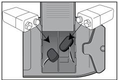
13 Insert the two 9V battery (included) into the compartment and slide the cover back on.
