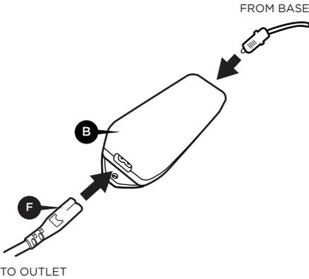
**7** Insert DC cord from base into the power supply.
