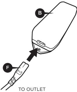
**6** Insert the AC cord into the power supply.
