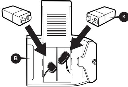
**12** Insert the two 9V batteries (included) into the compartment and slide the cover back on.
