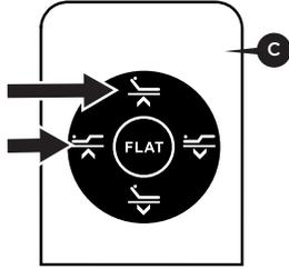
**14** Initial use of base requires additional run time. Simply press the Head Up button on the remote until the head section begins to lift. Then press the Foot Up button on the remote until the foot section begins to lift.
