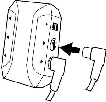
**5** Connect the Foot motor connector cable to control box.
