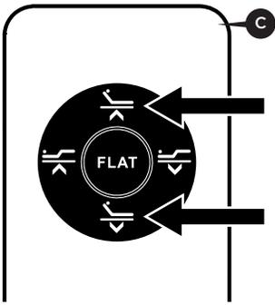
**2** Simultaneously press & hold the HEAD UP and HEAD DOWN buttons. When the LED light on the control box turns green, release the two buttons.
