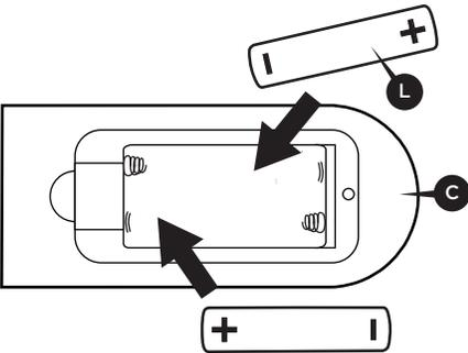
**10** Lift the battery cover and insert the two AAA size batteries (included) into the remote as shown in the figure. Replace the battery cover. Remote is already linked with the base.
