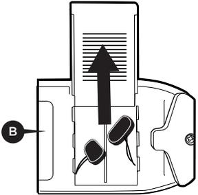
**11** Turn the power supply upside down to access the battery cover, then slide the battery cover off.
