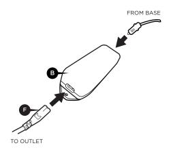
Insert DC cord from base into the power supply.
