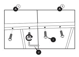
Secure the Base Pieces to each other using the eight hex bolts (four hex bolts for each Connecting Rod) making sure to hand tighten each and then tighten 1/4 turn more, as overtightening could cause damage to the frame or Connecting Rod.
