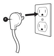
Insert AC plug into an AC outlet having 100-240V AC, 50/60Hz. Avoid outlets that work only with light switch.
