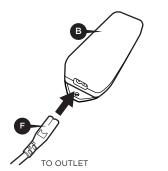
6 Insert the AC cord into the power supply.
