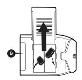
Turn the power supply upside down to access the battery cover, then slide the battery cover off.
