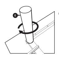
Insert the legs into the threaded holes at each corner of the base by inserting the leg and rotating clockwise until tight. There must not be any gap or wobble in the leg in order to avoid risk of injury or damage to the base which may void warranty.
