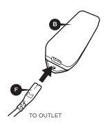
Insert the AC cord into the power supply.
