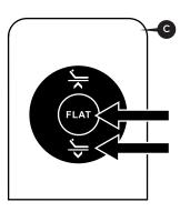
Simultaneously press & hold the FLAT and HEAD DOWN buttons. When the LED light on the control box turns off, release the two buttons.
