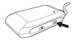
1 Double click the PAIR button on the control box (light will go on).
