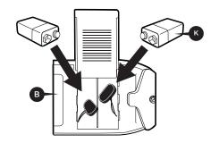
Insert the two 9V batteries (included) into the compartment and slide the cover back on.
