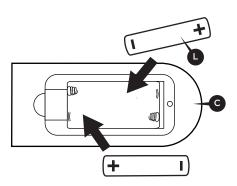
Diff the battery cover and insert the two AAA size batteries (included) into the remote as shown in the figure.
