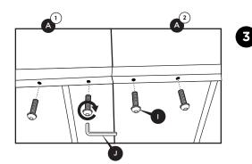
Secure the Base Pieces to each other using the eight hex bolts (four hex bolts for each Connecting Rod) making sure to hand tighten each and then tighten 1/4 turn more, as over-tightening could cause damage to the frame or Connecting Rod.
