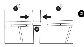
Insert the Connecting Rods into one of the Base Pieces and then slide the other Base Piece onto the Connecting Rods as shown.
