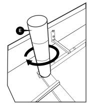
Insert the legs into the threaded holes at each corner of the base by inserting the leg and rotating clockwise until tight. There must not be any gap or wobble in the leg in order to avoid risk of injury or damage to the base which may void warranty.
