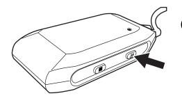
Double click the PAIR button on the control box (light will go on).
