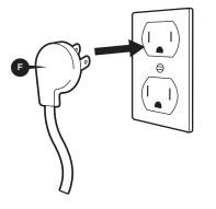
Insert AC plug into an AC outlet having 100-240V AC, 50/60Hz. Avoid outlets that work only with light switch.
