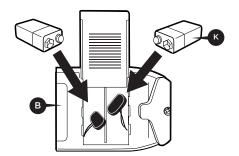
12 Insert the two 9V batteries (included) into the compartment and slide the cover back on.
