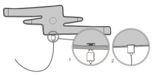
Insert the charger cable to the adaptor, and plug the charging adaptor into an electrical outlet.
