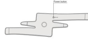
Turn the device ON by pushing the button located inside the Vibrant Logo on your device. Initial vibration will indicate that your device is ON and ready. After a short pause the 16 minutes treatment will start.
