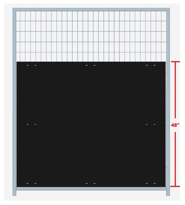
All the Isolation Panels are 48" tall. Install them with the 48" vertical and with the bottom edge sitting on the bottom frame and the back against the wire mesh. Equally space the small gaps on the left and right as needed.
