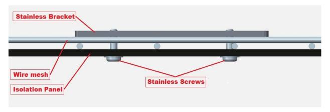
Install the stainless steel screws through the isolation panel and into the Stainless steel bracket which will sandwich the wire mesh in between the two. Leave the screw loose until they are all started, then tighten them from the bottom up on the isolation panel.
