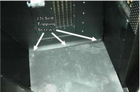
Once the front 3 screws are into secure, square the divider up in K9 insert and place 3 self tapping screws through the holes in flange into rear panel. Then 3 self tapping screws though the top into lid of K9 insert, and finally 3 self tapping screws into the floor through the rubber mat.
