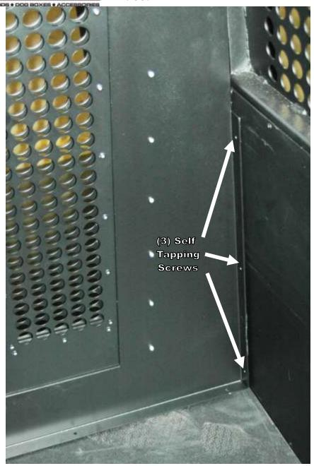
Place 3 self tapping screws in the flange on the divider located on the passenger side, start with the front into the front K9 insert.
