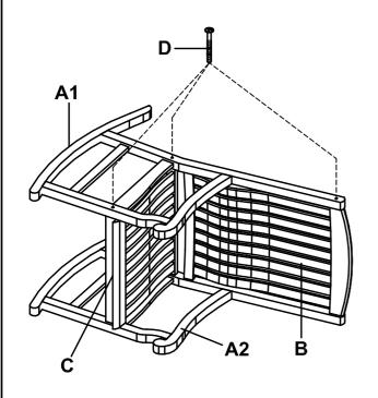
Invert the rocker and repeat step 2 procedure to secure frame.
