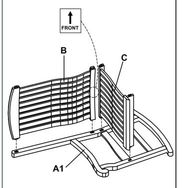
Attach back support (B) and seat (C) on to right side frame holes (A1). ( Apron with round edge must attached in front).
