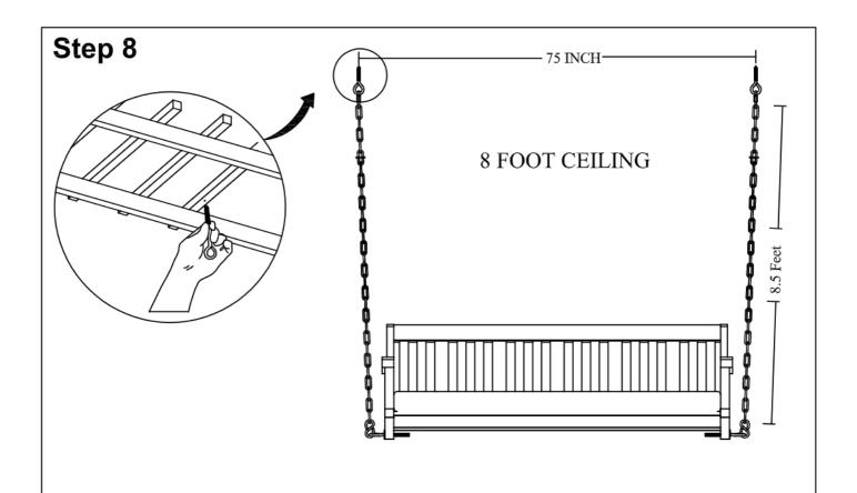
Attach the front hanger screws with a distance of 5 inches beyond the actual swing length (75 inches). then the 35 inch rear hanger screw. Mark the first two points the hanger screw will go. Next, measure the swing length plus 1-2 inches and mark the other two places. The next step, pre-drill pilot holes using Ø6mm drill bit size and attach the screw to the joist or beam.
