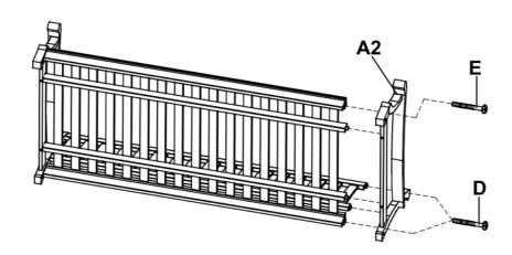
Attach Left side frame (A2) to the assembly from step 1, secure using 1 1/2" bolt (E) and Backrest (B) using 1 1/4" bolts (D).
