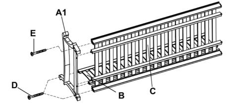
Attach backrest (B) and seat (C) into right side frame (A1). Secure Seat (C) using 1 1/2" bolt (E) and backrest (B) using 1 1/4" bolts (D).
