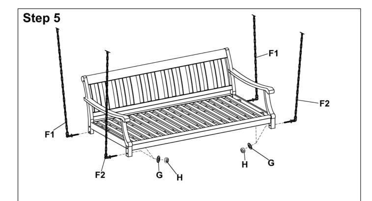
Install the chain with long bolt (F2) to front of side frame (A1 & A2), and chain with short bolt (F1) to the back of side frame (A1 & A2), secure using washer (G) and Nut (H), as diagram shown.
