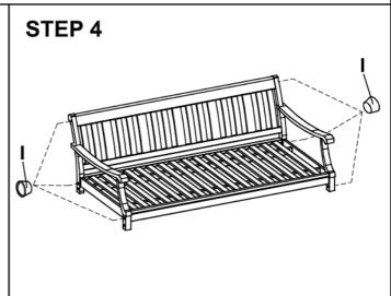
Tap in the wooden caps (I) to cover bolts head using rubber mallet.
