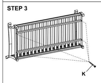
Secure seat (C) and side frame (A1&A2) using 1 3/4" screws (K). As shown.
