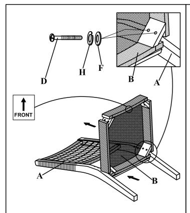
Attach the seat (B) to Back rest (A). Ensure the seat (B) align to the matching holes. Insert the small washer (F), spring washer (H) and 2" bolts (D) to the Attach the legs (C) into the seat (B). Secure it with big holes as shown in the diagram above. Adjust the bolts to the right position before screwing. Do not fully tighten the bolts yet.
