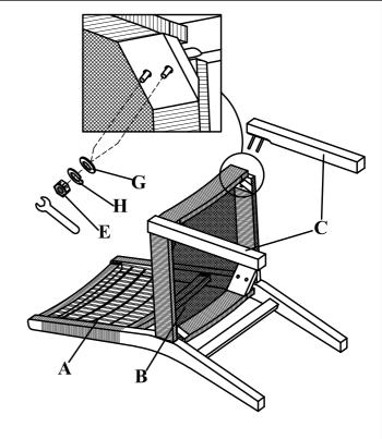
washer (G), spring washer (H) and nut (E). Tighten all bolts and nuts using screwdriver and wrench.
