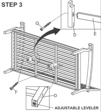
Attach the middle cross bar (E) into middle legs (D), secure using 2" bolt (G). Next, Attach the Middle Leg Frame to Seat, secure with 1 1/2" bolts (F), As Shown. Tighten all bolts using screwdriver.
