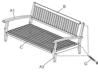
Attach back support (B) and seat (C) Into right side frame (A1), secure using 2" Bolts (G). Tighten all bolts using screwdriver.
