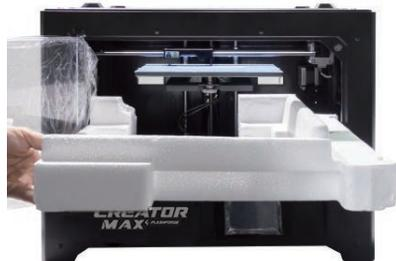
10. Take the bottom protective foam from the printer and then lower the build plate back.
