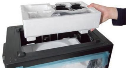
5. Remove the foam container. It should contain: power cable, USB cable, two spool holders, SD card, tool bag, extruder's accessory kit, one 1kg red pla filament.
