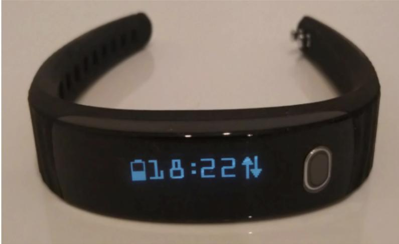
1. When the display of the Bracelet shows X it means that it is not connected to the Phone.
