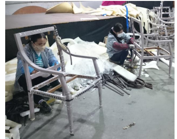
Paper is reinforced with wrapping
