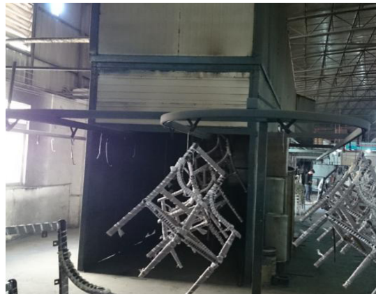
Chairs are rotated on the heat line for 2-3 hours
