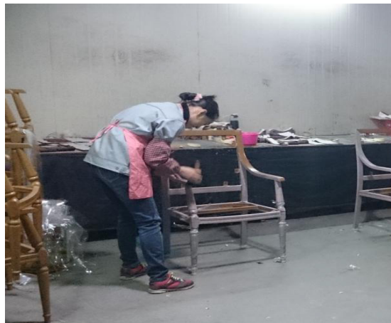
Paper is adhered to the frame
