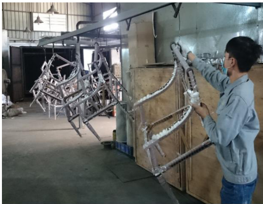
Chairs are added to the auto heating line
