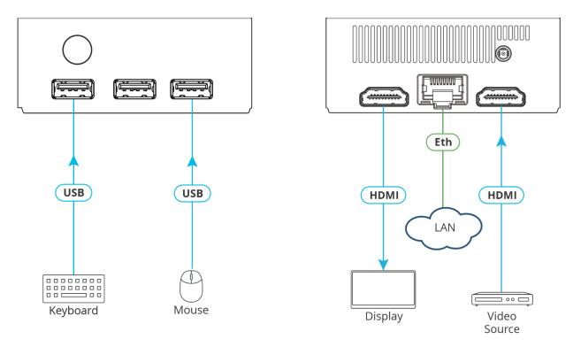
Figure 5: Connecting VIA Connect<sup>2</sup>
