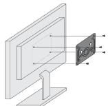
1. Attach the VESA mounting bracket 2. Fasten two screws to the bottom to the back of the display with 4 screws.
