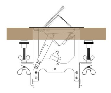
**C**: Connect the power cable from underneath the **TBUS-204** and then power or charge devices as required.
