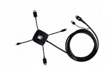
KSPIDER is an active multiformat male input to HDMI male output adapter that enables you to connect one HDMI, DisplayPort, mini DisplayPort, or USB TypeC source to an HDMI acceptor
