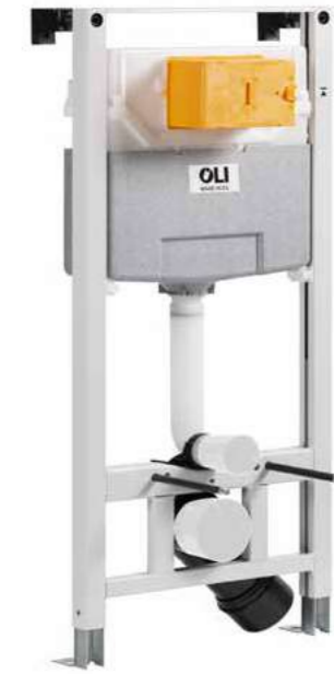
1200cm Pre-wall, freestanding w.c frame including brackets and w.c bend with 3/6 litre dual flush plate, front flush installation only.
