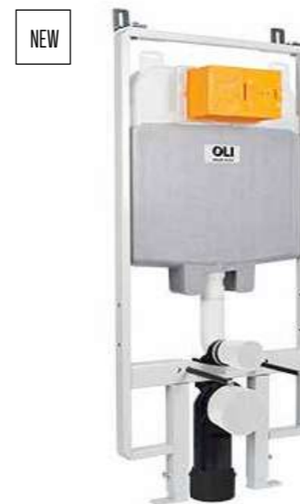
1200cm Slim Pre-wall, freestanding w.c frame including brackets and w.c bend with 3/6 litre dual flush plate, front flush installation only.
