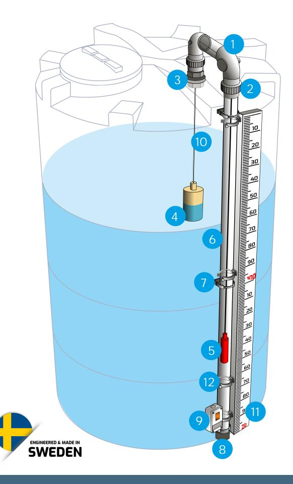
90° pulley elbow made from PVC available in both 40 mm and 1.25" Manufactured
