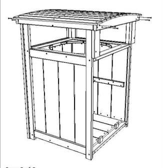
5. Keep top of removable Back Panel tilted back & align bottom blocks, tilt top forward & insert pins through top Rim.
