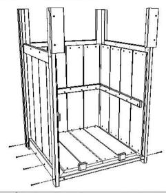
3. Align Top Rim with all top crosspieces. Keep Pin Holes on back Side. Install 4 - 2" Screws Per Side Panel in predrilled holes then install 6 - 2" Screws in predrilled holes in front Panel.
