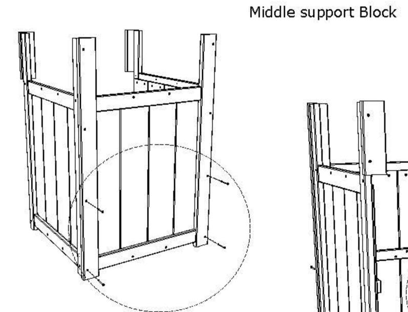
Note: Only attach bottom 2 Screws on each side as shown.
