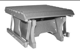
STEP #6 - Attach the Top Assembly to the Glider Brackets and secure with 4- 5/16" Lock Nuts. (See Glider Bracket Diagram.)
