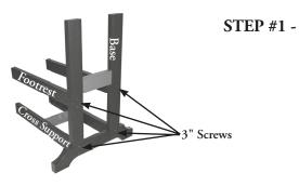
First, assemble the cross support to the base using 3" screws. Second, fasten the footrests to the base using 3" screws (Bar and Counter Height Only.)
