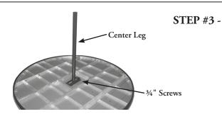
Position the center leg over the umbrella plug and fasten the center leg to the top using <sup>3</sup>/<sub>4</sub>" screws. **Caution! To keep screws from spinning out, do not overtighten screws!**
