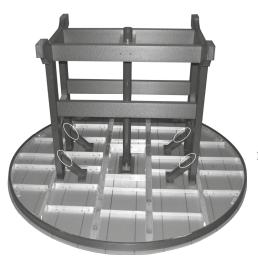
STEP #5 - Last, attach the Braces to the Top and the Base using 1½" Screws and 5/8" Pan Head Screws (these go into the top).
