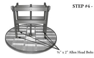
STEP #4 - Lift the base assembly onto the top. Fasten the base assembly to the aluminum frame using 1/4" x 2" Allen Head bolts.
