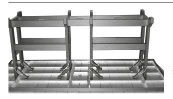
STEP #5 - Last, attach the Braces to the Top and the Base using 1½" Screws and 5/8" Pan Head Screws (these go into the top).
