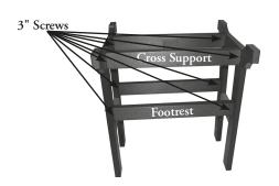
**STEP #1** - First assemble both Bases and Long Cross Supports using 3" Screws.
