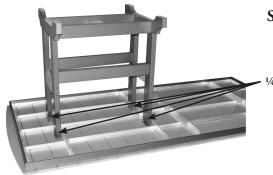
STEP #2 - Attach the first Base Assembly to the aluminum frame of the Top using 8- 1/4" x 2" Allen Head Bolts.
