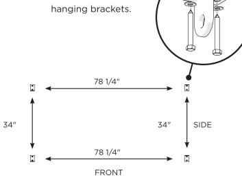
**NOTE:** Dimensions of the hanging brackets are to the center of the brackets.
