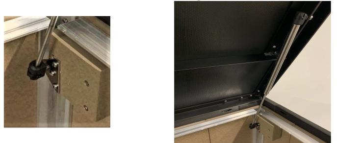
Have one person hold open the lid while a second person pushes the bottom of the cylinder onto bracket until you feel it click into place. To ensure it is properly secured make sure you can not remove the cylinder by pulling backwards on it. Push the top of the cylinder onto the bracket that is attached to the aluminum frame and ensure it is properly secured. Repeat on opposite side. Your Cushion Storage Box is now complete! NOTE: *Bottom half of cylinders are thinner than top half.*
