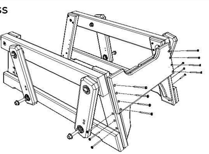
2. Attach (E) Back Cross Pc. to Glider Base Sides using 7 - 2" Screws per side, Be sure to match all numbers & letters.
