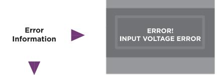
**ERROR!** INPUT VOLTAGE ERROR Input voltage is higher than 18V, check the power supply, then restart the charger.
